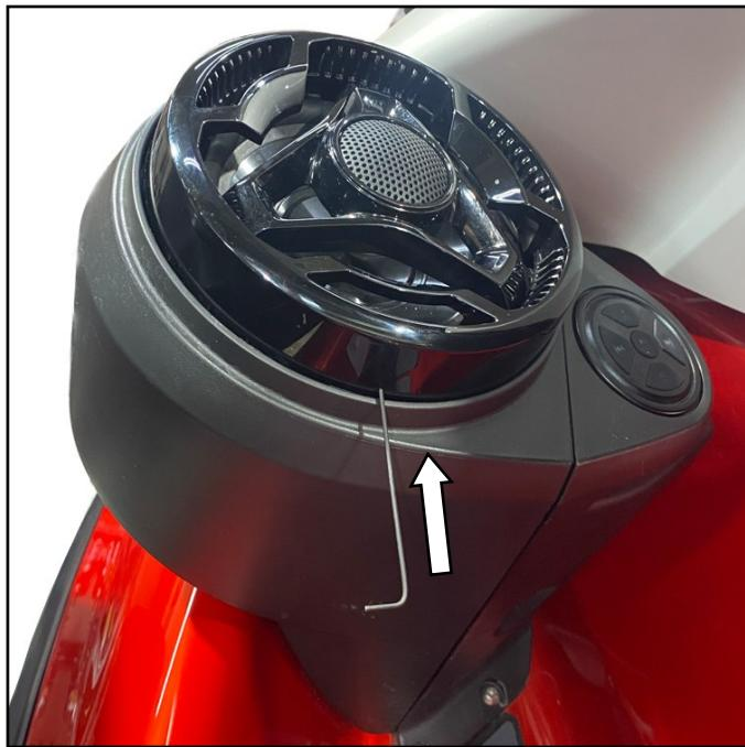
Using a T-20 Torx bit, remove Torx screws (6) securing each factory speaker to its speaker pod .
