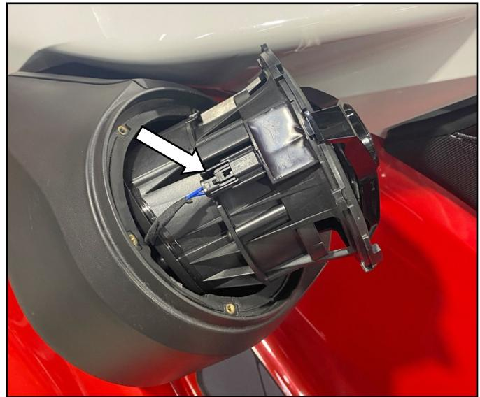
Connect wire harness adapters to factory speaker wires in each speaker pod, **NOTE: Apply dielectric grease onto end of factory connectors. Ensure connectors 'lock' together.**
