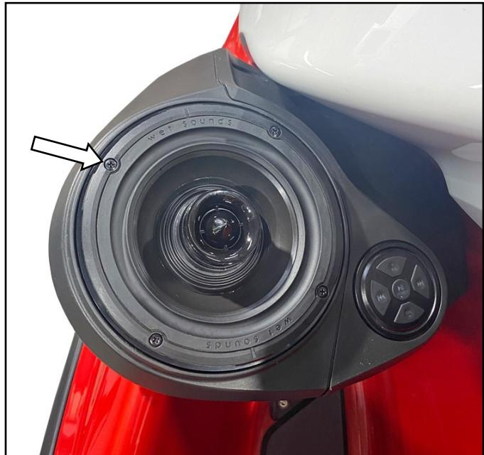
Secure adapter rings to speaker pods using factory Torx screws (6 per adapter ring). **NOTE: Apply blue Loctite to screws. Do not overtighten.**
