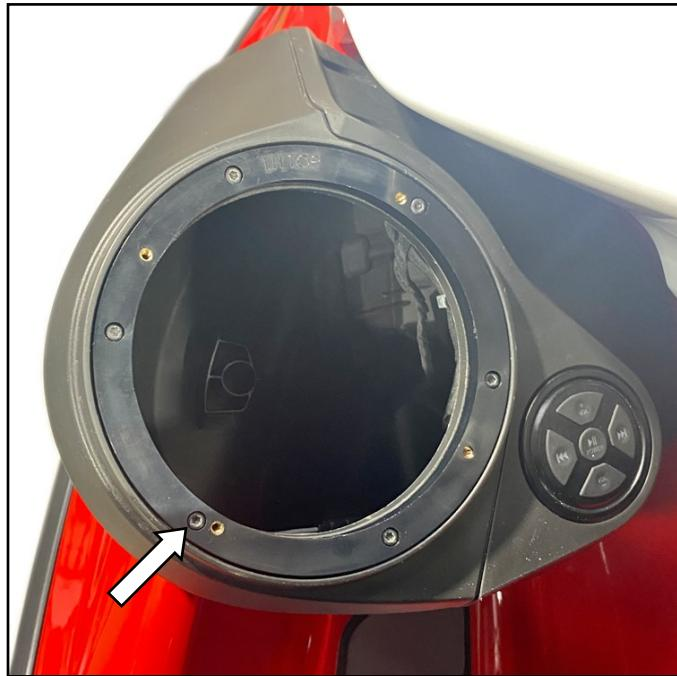
Insert supplied speakers into factory speaker pods. Secure speakers to adapter rings using supplied Phillips head screws (4 per speaker). **NOTE: Apply blue Loctite to screws. Do not overtighten.**
