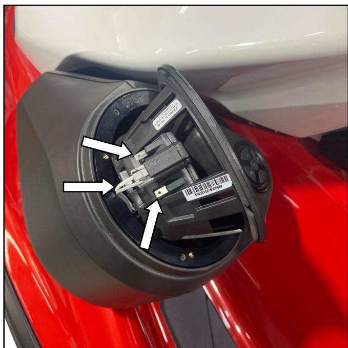
Identify locking tabs on inner edge of supplied speaker grills and outer edge of supplied speakers (6 each).
