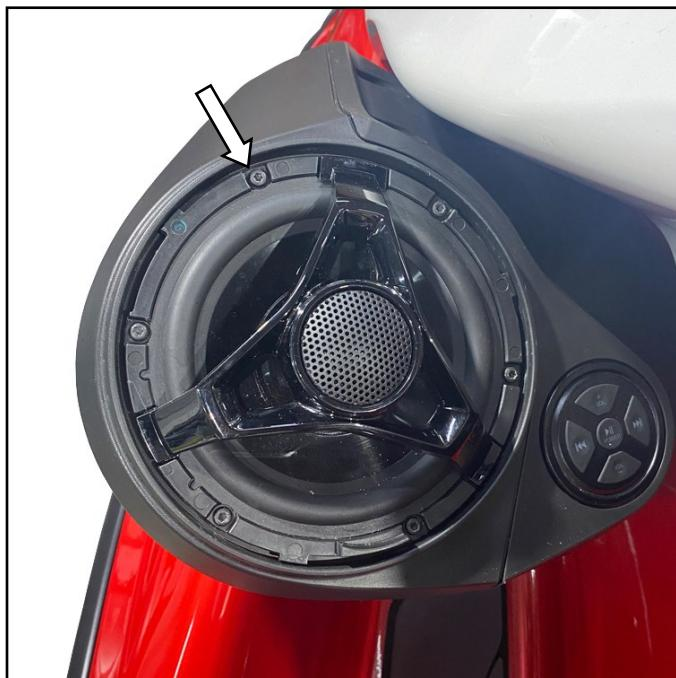
Carefully remove each speaker and disconnect electrical connector.
